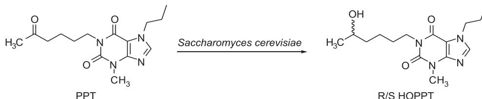
Fig. Bioreduction pathway of propentofylline by yeast.
